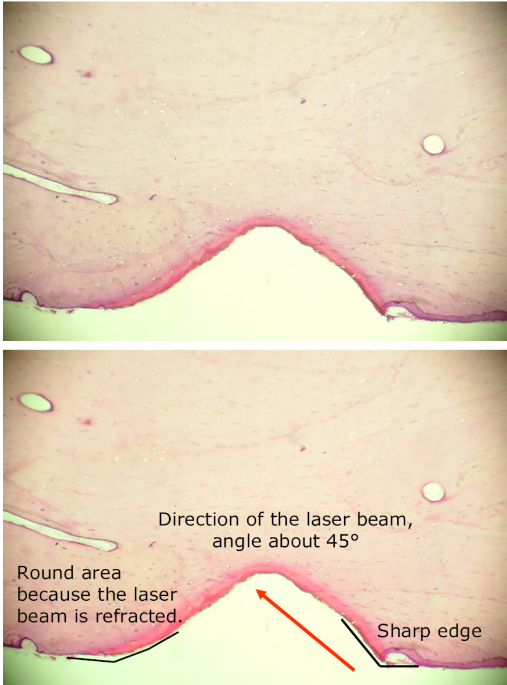
Fig. 36 a and b: A1/1 – Magnification factor 10 x (and explanation)
